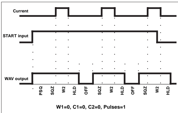
Figure 7-3. Repeat Spot Weld
